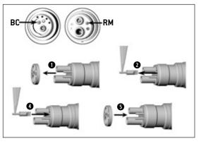
Cleaning/Replacing the water filter RQ-53 / RQ-54 TE-95 BC / RM, TE-97 BC / RM, TE-98 BC / RM
